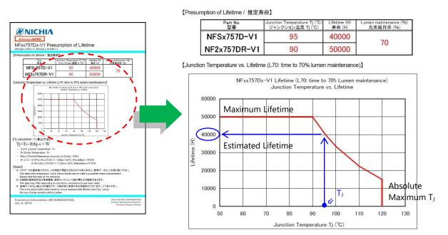
Figure 3. Example of the Technical Data (NFSx757D-V1/NF2x757DR-V1 Presumption of Lifetime) This document contains tentative information, Nichia may change the contents without notice.
