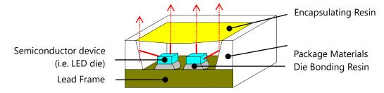
Figure 2. Internal Structure of a NICHIA 757 series LED
