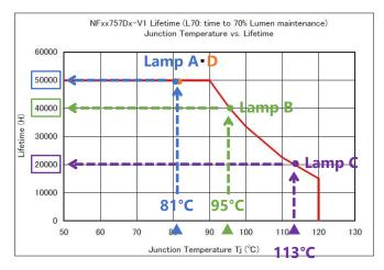
Figure 6. Lifetime Estimation of Selected LED Retrofit Lamps
